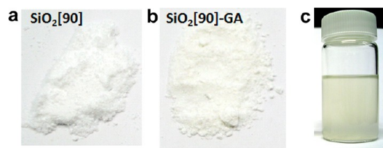
Figure 2. (a) Untreated and (b) functionalized SiO 2 [90]-GA NPs. (c) Suspension (5 mg of SiO 2 [90]-GA NPs in 10 mL of methanol).
